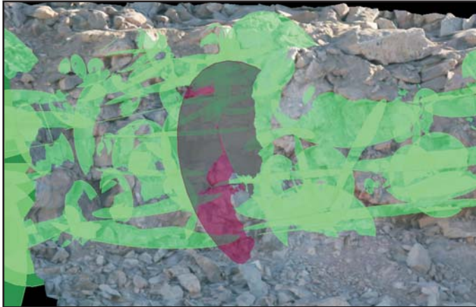
Bench fabric mapping using Adamtech's 3DM software
